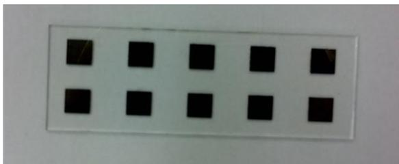
Fig. 4. Glass substrate with printed structure by ink1
