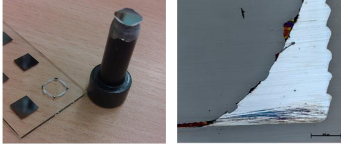
Fig. 5. Samples printed by ink1 on glass after pull-off test
